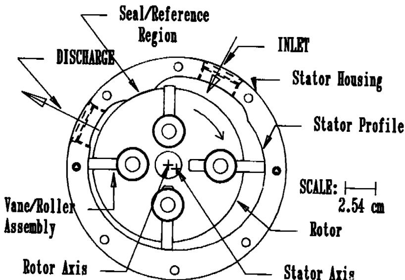
FIGURE 3: Frontal Assembly Drawing of the ROVAC Model 230 CRV Machine
