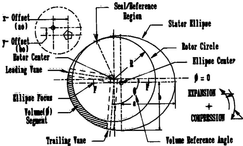
FIGURE 2: Stator/Rotor Geometry of the CRV Machine
