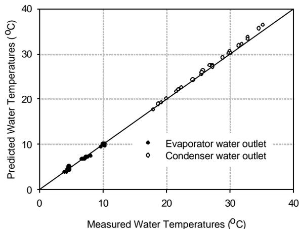
Fig. 4: Steady state leaving water temperatures
