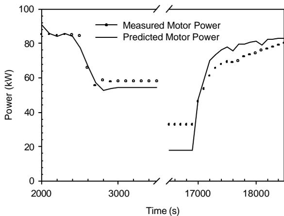
Fig. 9: Transient motor power
