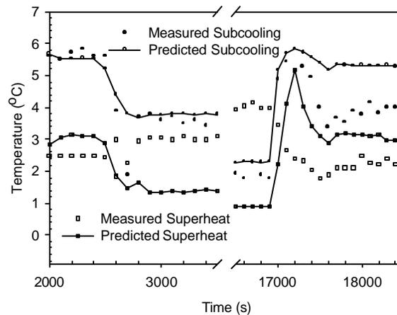
Fig. 10: Transient sub-cooling & superheat
