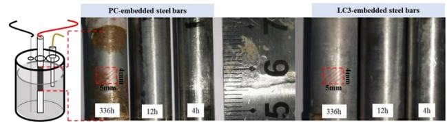
**Figure 7.** Photographs of embedded steel bars in PC and LC3 pastes for various ages of hydration (shade area refers to XPS specimens)
