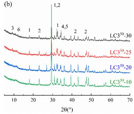
**Figure 6.** XRD patterns of curing age of 3d, (a) standard curing, (b) steam curing (1-calcium carbonate, 2-calcium hydroxide, 3-Ettringite, 4-Dicalcium silicate, 5-Tricalcium silicate, 6-Carboaluminat.)
