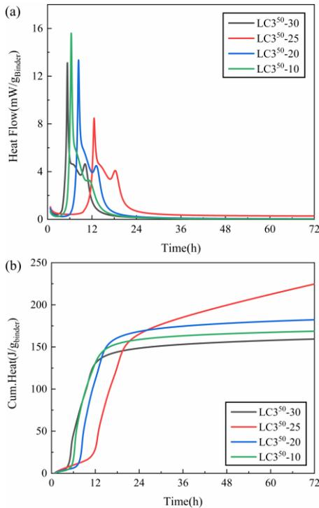
**Figure 8.** The hydration heat of steam curing, (a) hydration heat release rate, (b) cumulative heat release.
