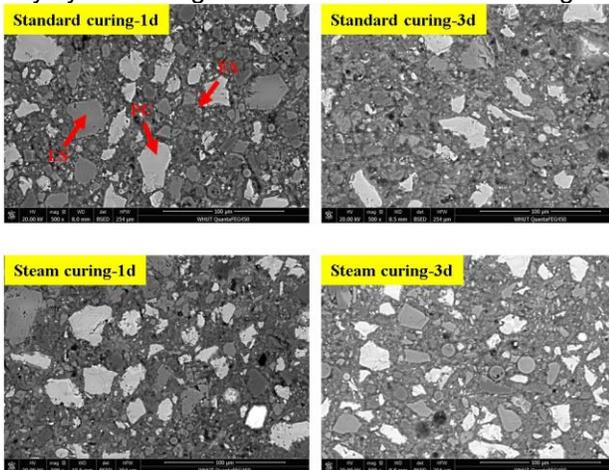
**Figure 9.** LC<sup>3</sup>50-30 standard curing and steam curing 1d and 3d SEM-BSE images
