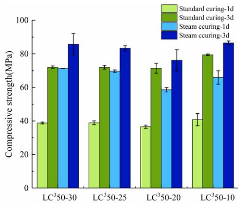
Figure 3. 1d and 3d compressive strength
