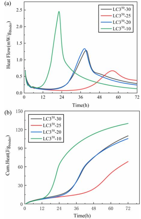
**Figure 7.** The hydration heat of standard curing, (a) hydration heat release rate, (b) cumulative heat release.
