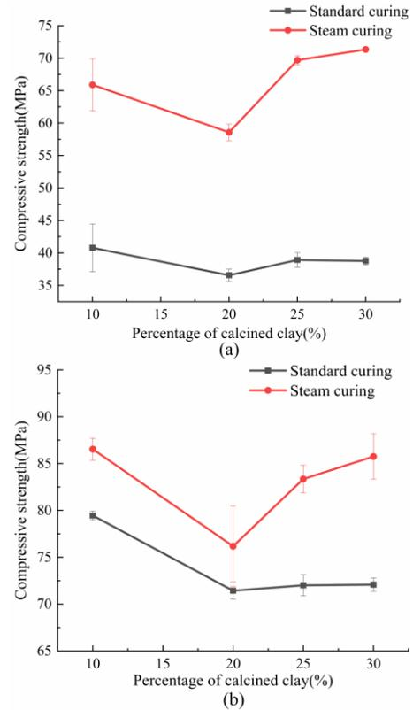
Figure 4. The 1d and 3d compressive strength changes with the ratio of calcined clay / limestone, (a) curing age of 1 d; (b) curing age of 3 d.
