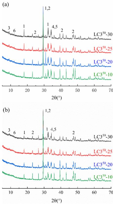
**Figure 5.** XRD patterns of curing age of 1d, (a) standard curing, (b) steam curing (1-calcium carbonate, 2-calcium hydroxide, 3-Ettringite, 4-Dicalcium silicate, 5-Tricalcium silicate, 6-Carboaluminat)
