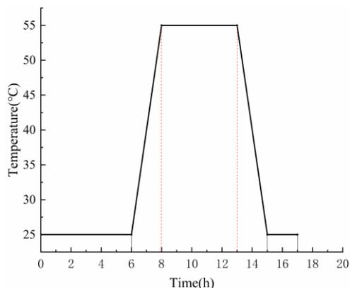
Figure 2. Steam curing system
