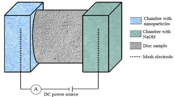
**Figure 2.** Electro-migration chamber used for ionic exchange test
