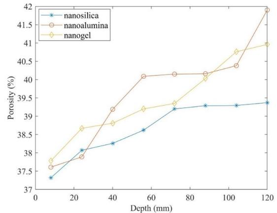
**Figure 6.** Porosity changes along the direction of injection
