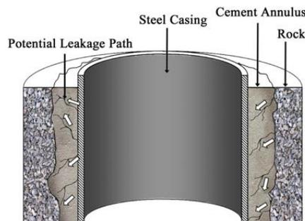
Figure 1. Possible leaking paths for gas
