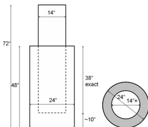
**Figure 4.** Casting hollow cylinders
