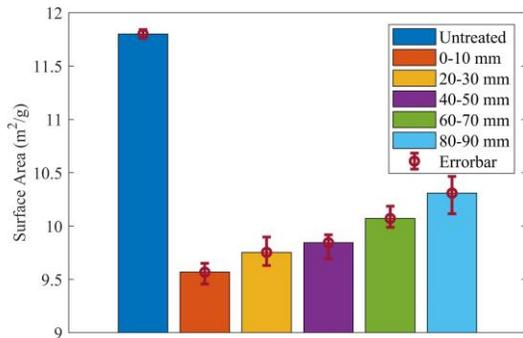
**Figure 5.** Surface area of pores of noninjected sample at different depths
