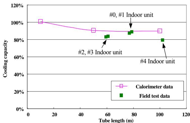
Figure 2 : Effect of tube length and head on cooling capacity
