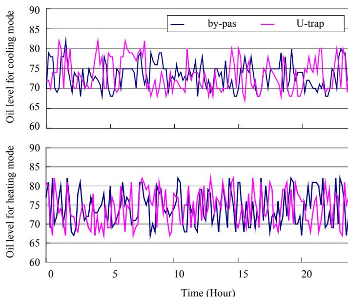
Figure 7 : Oil levels with and without oil U-traps
