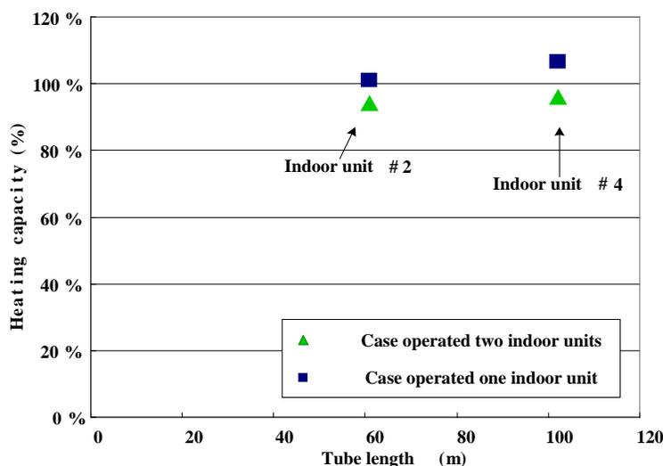
Figure 5 : Effect of head between adjacent indoor units on the heating capacity
