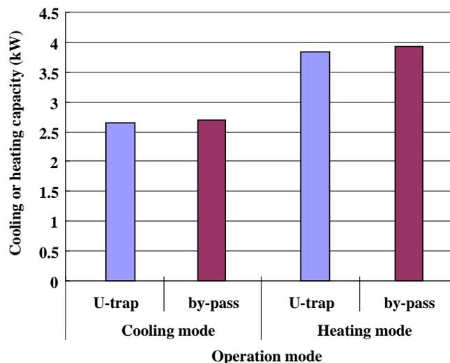
Figure 8 : Comparison of cooling and heating capacities for the cases with and without U-traps
