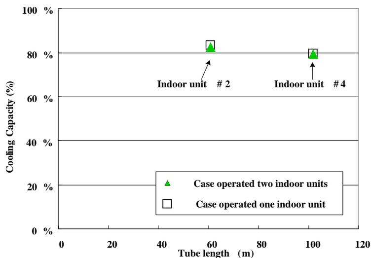
Figure 4 : Effect of head between adjacent indoor units on the cooling capacity
