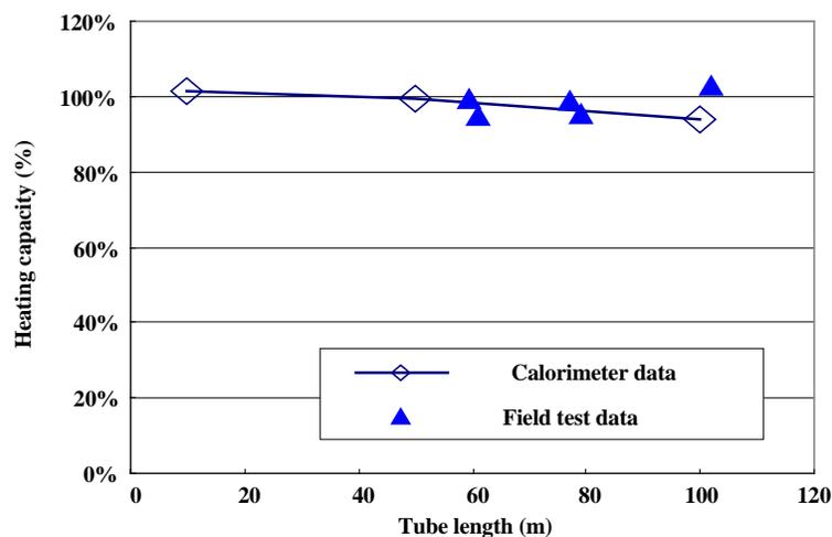
Figure : 3 Effect of tube length and head on heating capacity
