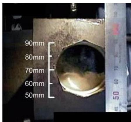
Figure 6 : Visualization of oil level in the scroll compressor
