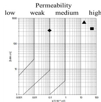
Fig. 3. Air permeability of the panel 50 meters from the South entrance.
