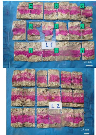
**Fig.5.** Carbonation depth on cylinders 50 meters (left) and 150 meters (right) from the South entrance.
