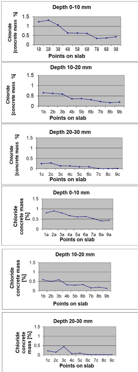
**Fig. 6.** Chloride content on the 50 meters (left) and 150 meters (right) wall panels at different depths.
