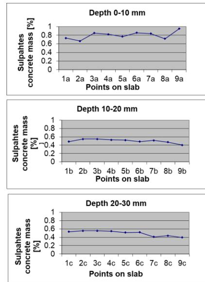
**Fig. 7.** Sulphate profiles on the concrete wall panel 50 meters inside the tunnel, measured down to a depth of 30 mm.
