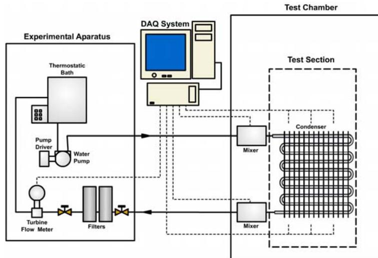
Figure 1: Experimental apparatus
