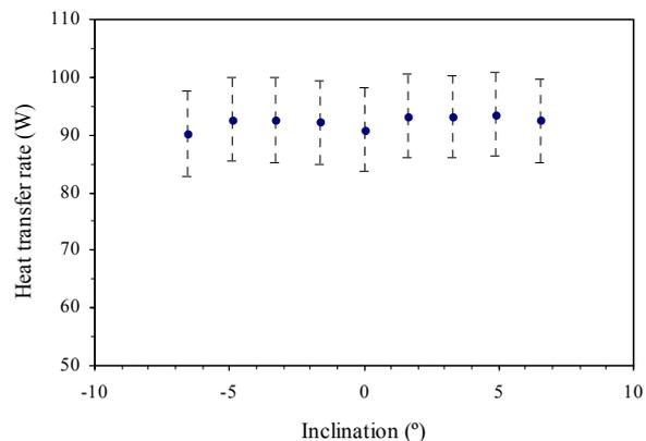
Figure 7: Effect of the inclination of the heat exchanger
