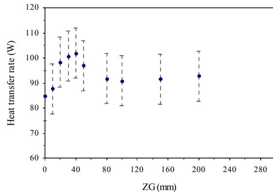
Figure 6: Effect of the gap between the refrigerator and the side walls
