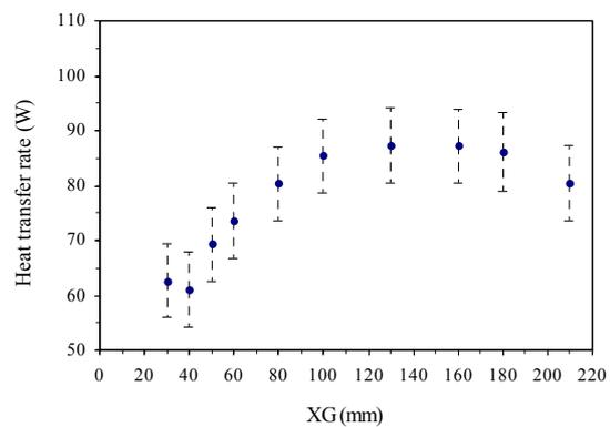
Figure 3: Effect of the gap between the refrigerator and the rear wall
