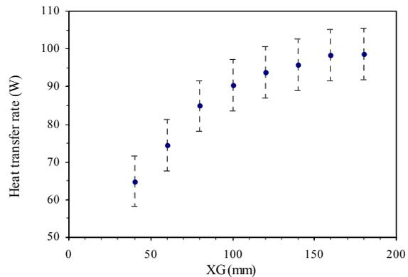
Figure 5: Effect of the gap between the refrigerator and the rear wall
