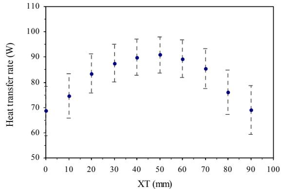
Figure 4: Effect of the gap between the heat exchanger and the rear wall
