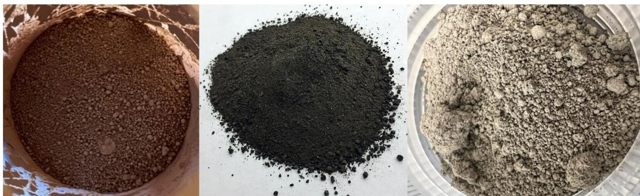
**FIGURE 4.** Images of bulk aerosol dusts used in this work. Left: Arizona Test Dust (ATD) simulant dust. Middle: Image of Johnson Space Center lunar mare simulant (JSC-1A) created at NASA (Cannon, 2023). Right: Exolith Mare LMS-1D simulant dust.
