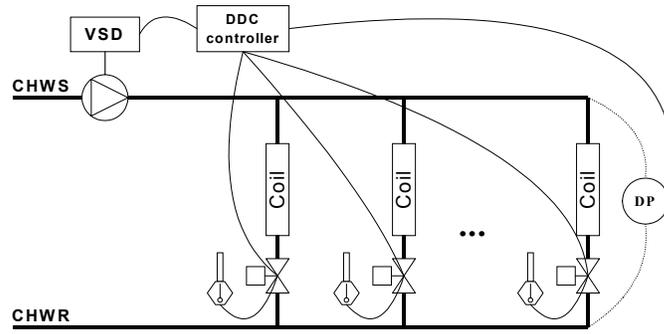
Figure 1. Typical chilled water distribution system
