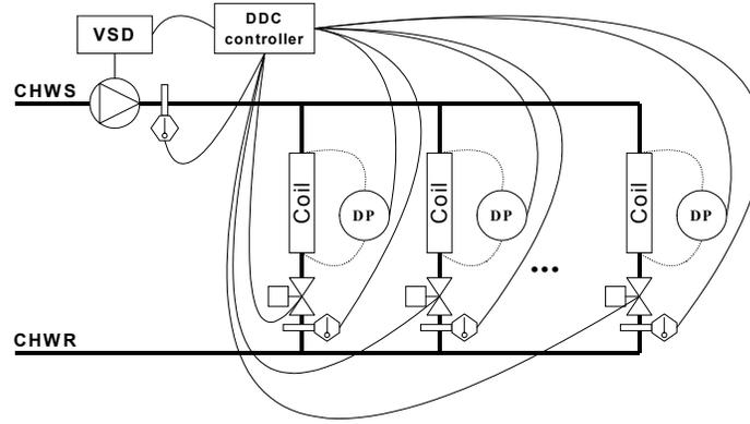
Figure 2. Proposed chilled water distribution system
