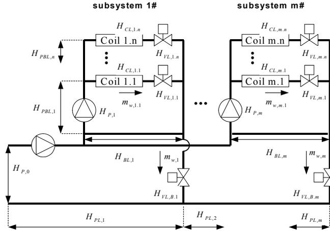
Figure 4. Primary-secondary-tertiary pumping system
