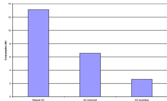
Figure 4 – Energy consumption of fan technologies.
