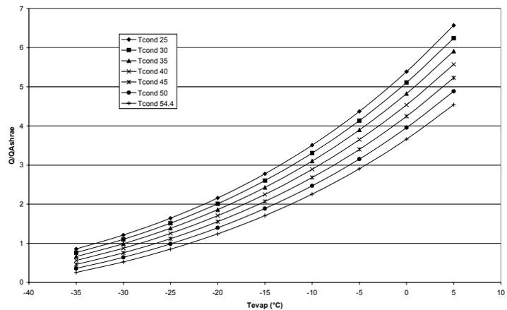
Figure 2 – Cooling capacity at different evaporating and condensing temperatures.
