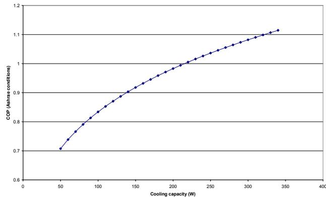
Figure 3 – COP ASHRAE variation with the cooling capacity.
