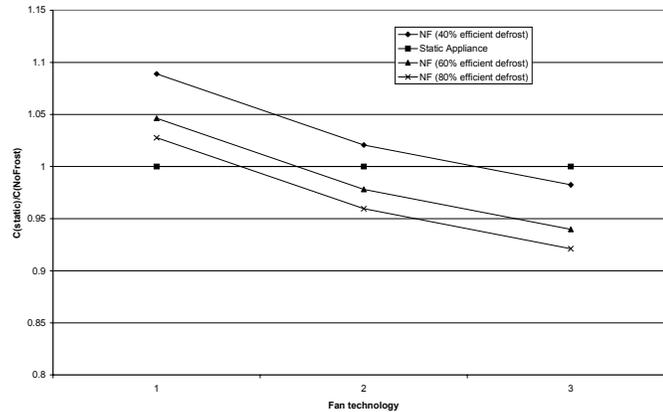
Figure 5 – Consumption of the no-frost appliance relative to the static appliance.
