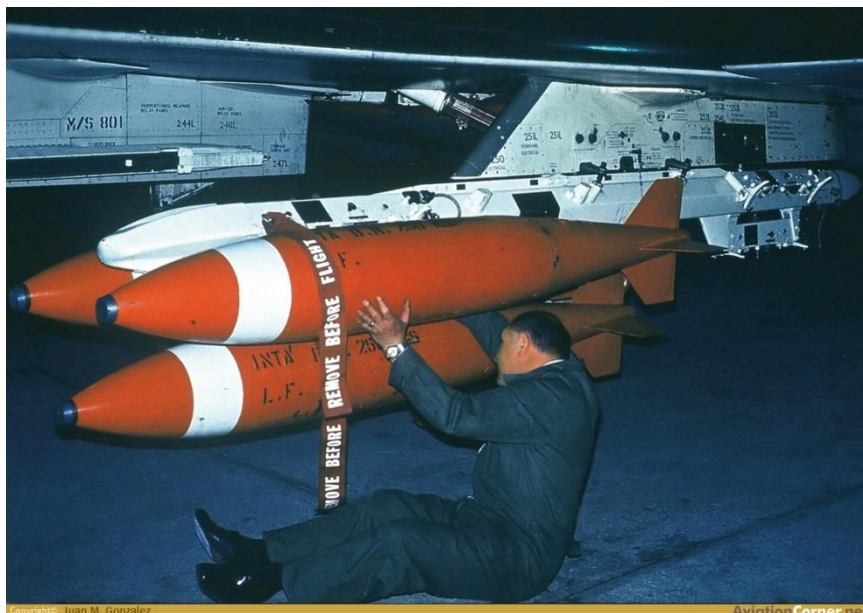
Figure 12: Multiple Ejection Rack attached to an F-4 Fighter from Aviationcorner.net
