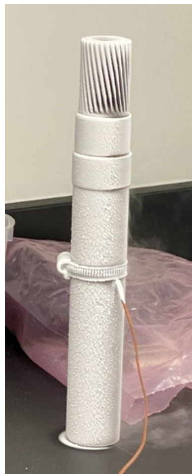
Inner component after being submerged in liquid nitrogen.
