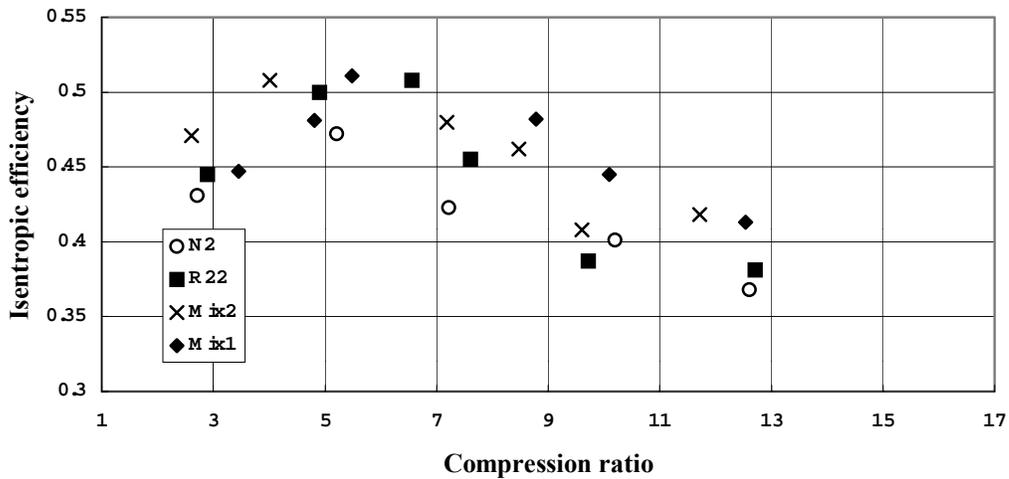
Figure 2. Test data on the isentropic efficiency for 4 cfm reciprocating hermetic compressor.
