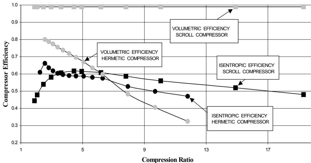
Figure 4. Efficiencies of large reciprocating hermetic and scroll compressors designed for R404a.
