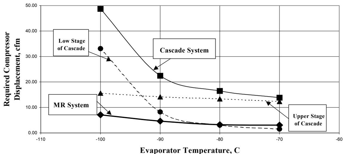
Figure 5. Actual Systems with reciprocating hermetic compressors.
