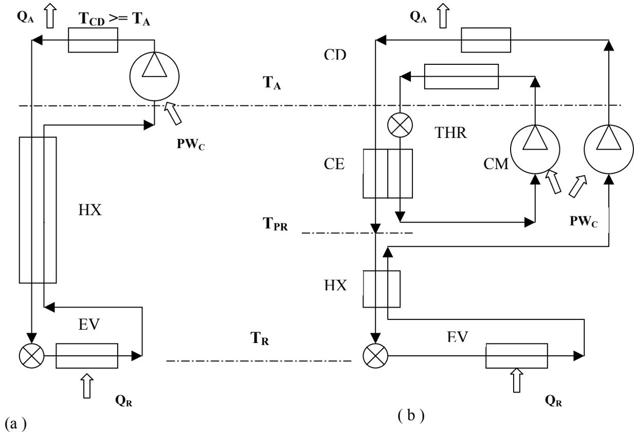
Figure 1. Schematics of the cascade and MR cycles.
