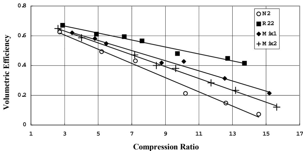
Figure 3. Test data on the volumetric efficiency for 4 cfm reciprocating hermetic compressor.
