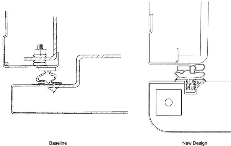
**Figure 5: Baseline and New-Design Perimeter Face Frame Cross Sections**
