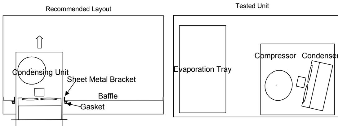
**Figure 4: Condensing Unit Layout for Tested Beverage Merchandiser and Recommended Modification**
