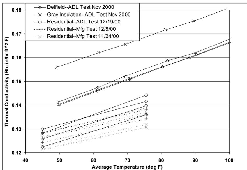
**Figure 2: Thermal Conductivity Measurements**
