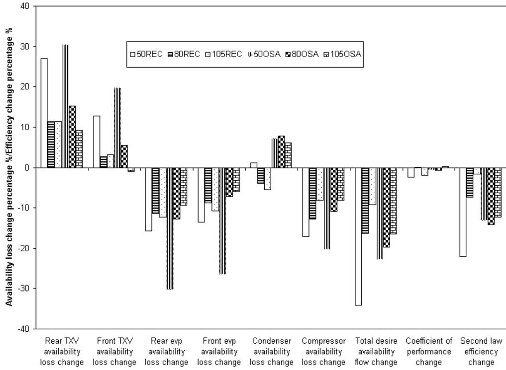
Figure 5: Availability Loss And Efficiency Comparison Between New And Base Systems.
