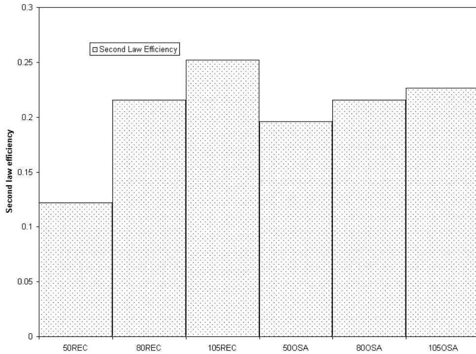
Figure 4: The Baseline A/C System Second Law Efficiency.
