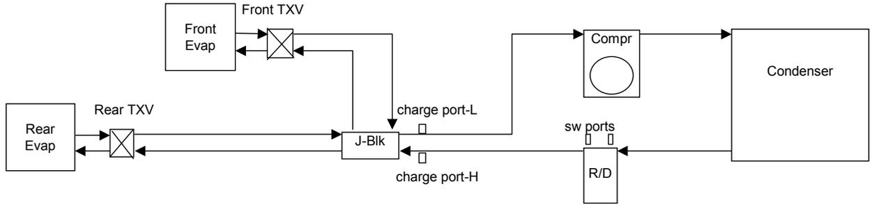
Figure 1: Vehicle A/C System Schematic
