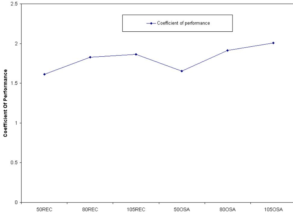
Figure 3: The Baseline A/C System Coefficient of Performance.
