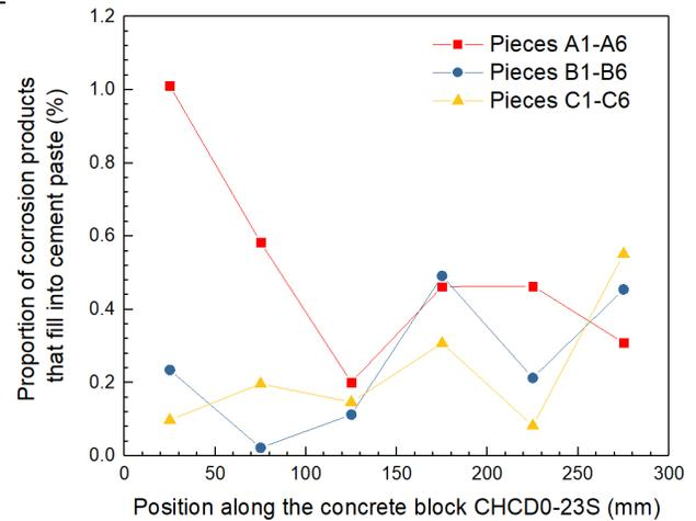
**Figure 11.** The proportion of corrosion products filling into the cement paste to the whole steel bar
