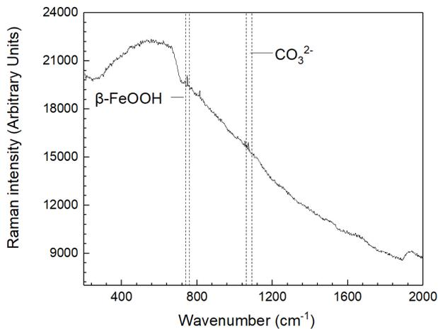
**Figure 6.** Raman spectra of the solution in simulated aggressive environment
