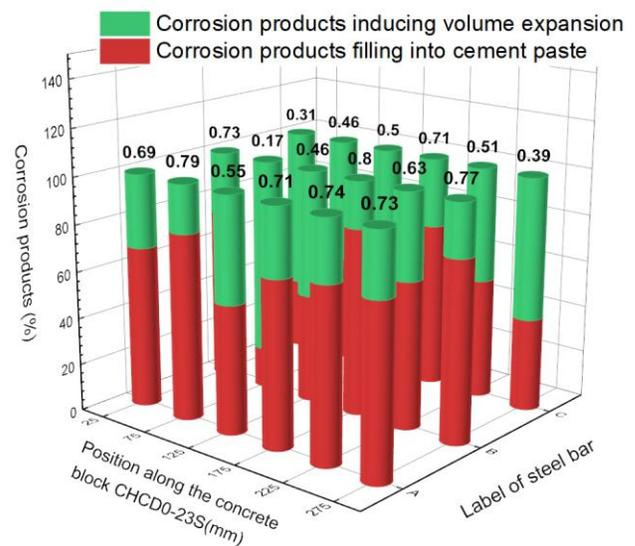
Figure 12. The proportion of corrosion products filling into the cement paste and corrosion products inducing volume expansion
