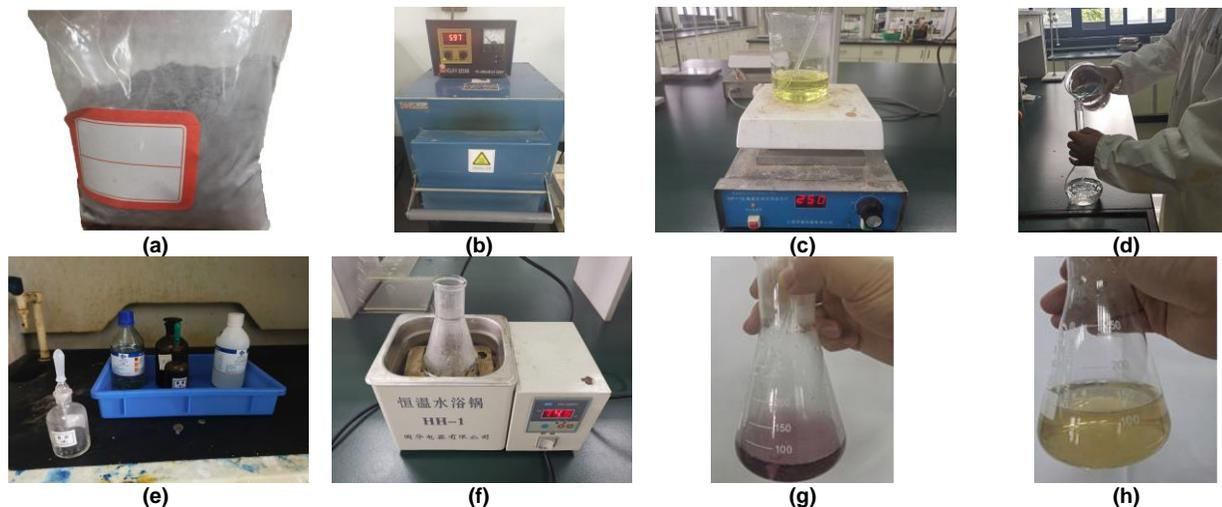
**Figure 5.** Process of titration (a)concrete powder (b)muffle furnace (c)leaching out dissolved in HCl and HNO<sub>3</sub> (d)bring to volume (e)adjust PH in fume hood (f)heat in water bath for titration (g)add sodium sulfosalicylate to sample solution before titration (h)titration end point
