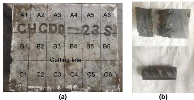
**Figure 3.** Cut process of sample preparation (a)cutting line on concrete block (b)seperated concrete parts and steel bar segment of each piece
