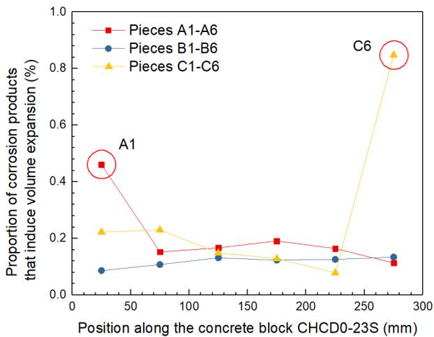
**Figure 10.** The proportion of corrosion products inducing volume expansion at steel-concrete interface to the whole steel bar
