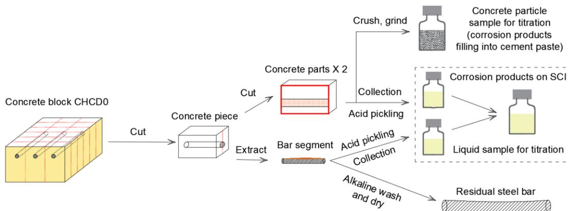
**Figure 4.** Process of sample preparation
