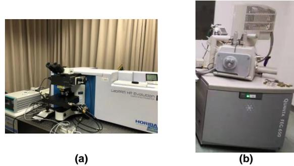
**Figure 2.** Equipment used in the experiments (a)Raman spectroscopy (b)scanning electron microscope
