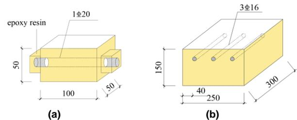
**Figure 1.** Scheme of specimens(a)mortar block (b)concrete block of HangZhou Bay Bridge
