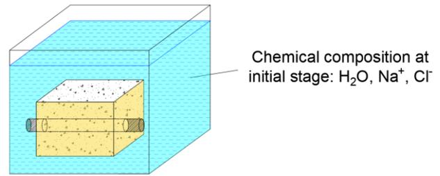
**Figure 7.** Chemical composition of solution in simulated aggressive environment
