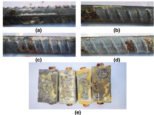
**Figure 8.** Mortar blocks(a)M-0.5-10 (b)M-0.5-15 (c)M-0.65-15 (d)M-0.5-20 (e)blocks after wet-dry cycle
