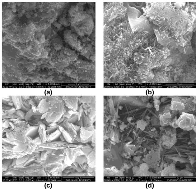
**Figure 9.** SEM image of corrosion products (a)ferrihydrate (b)goethite (c)hematite (d)akaganeite
