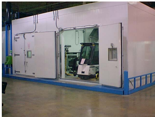
Figure 1: MCC Calorimetric Testing Facility
