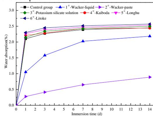
**Figure 1.**Water absorption of concrete coated with different impregnating agents
