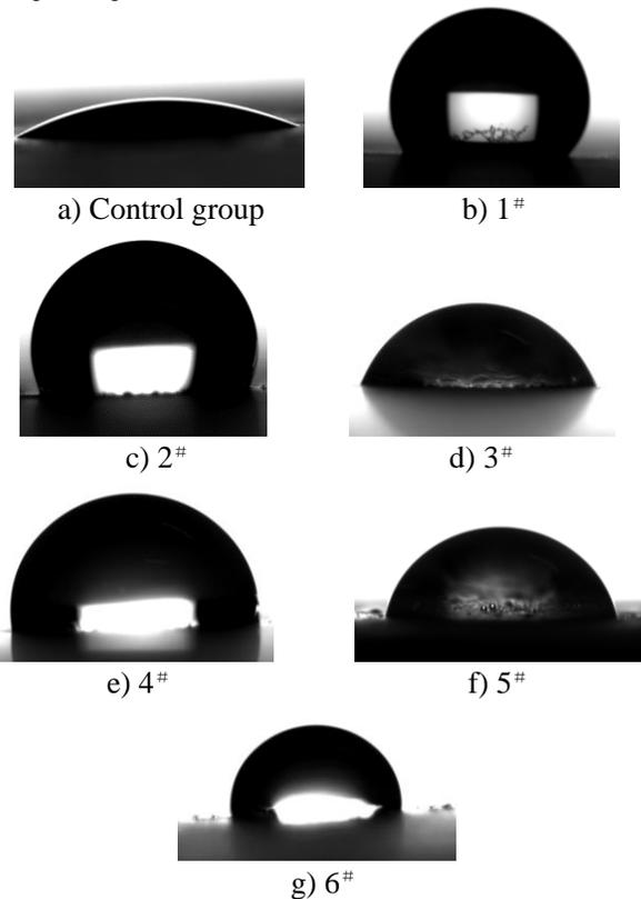
Figure 4. Contact angle of concrete surface coated with different impregnate agents
