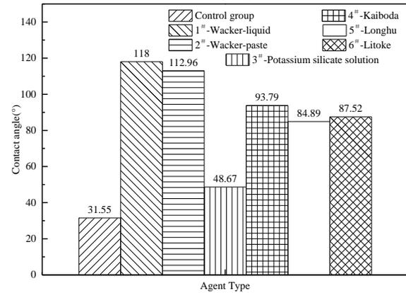
Figure 3. Contact angle of concrete coated with different impregnate agents
