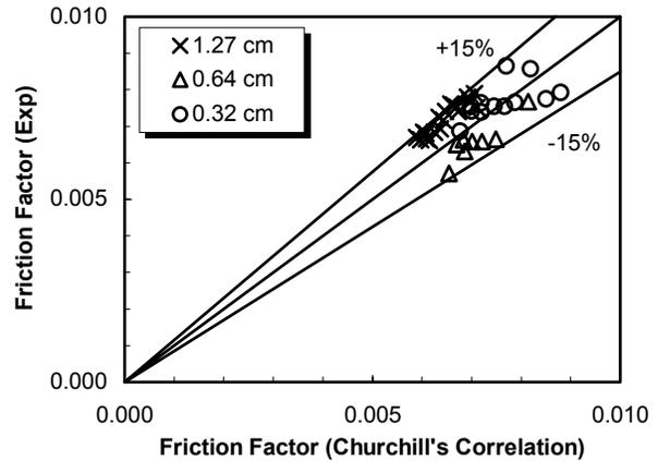
Figure 3. Experimental Vs. Churchill's Friction Factors (Air Flow)
