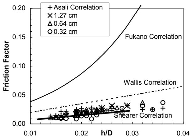
Figure 4. Friction Factor Vs. Dimensionless Mean Film Thickness  $h/D$  (Air/Oil Flow)
