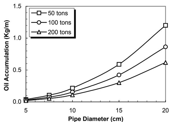
Figure 8. Prediction of Oil Accumulation in Different Size Pipes (0.5% Oil)
