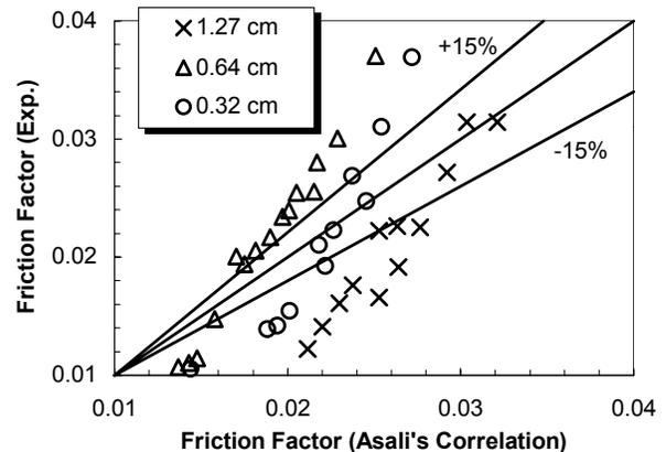
Figure 5. Experimental Vs. Asali's Friction Factors (Air/Oil Flow)
