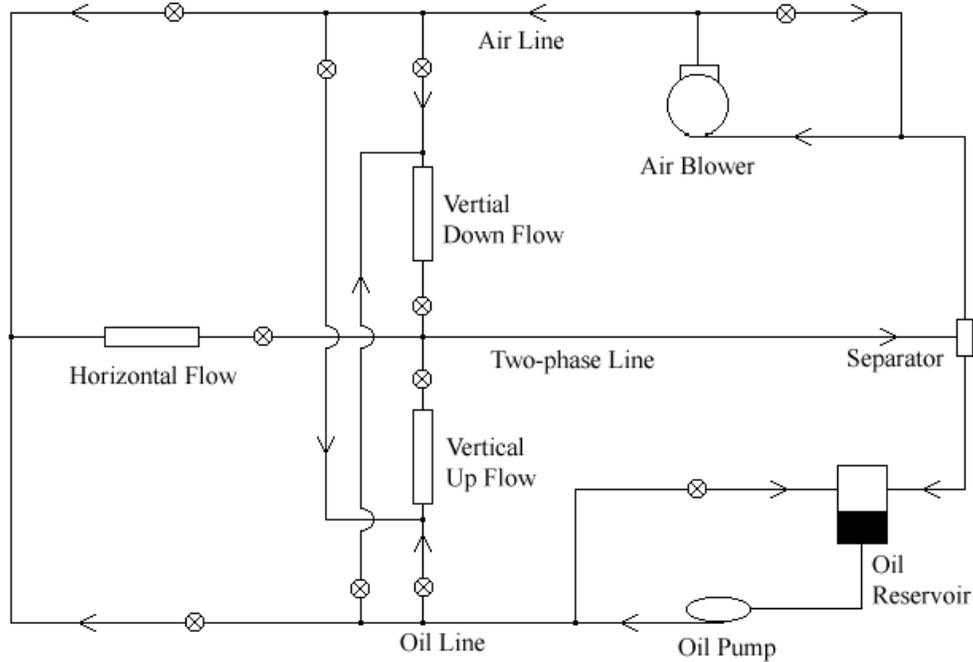
Figure 1: Schematics of Flat Plate Experimental Apparatus
