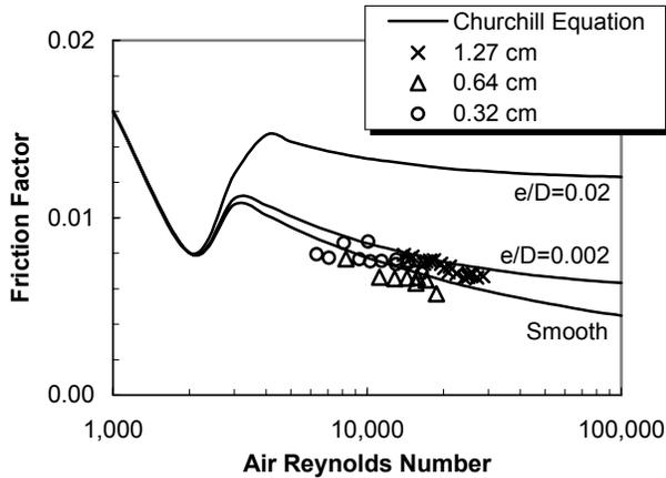
Figure 2. Friction Factor Vs. Air Reynolds Number (Air Flow)
