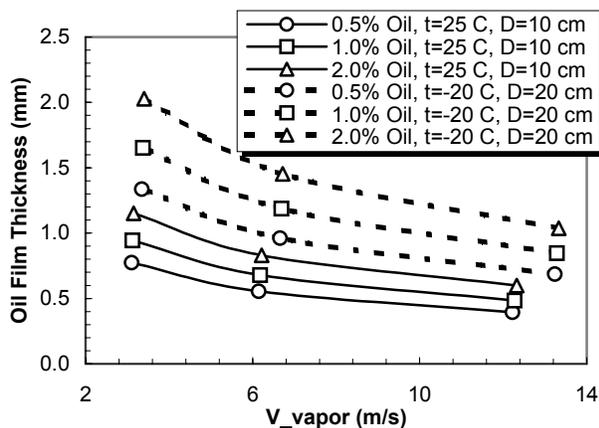
Figure 7. Prediction of Oil Film Thickness with Shear Stress Model
