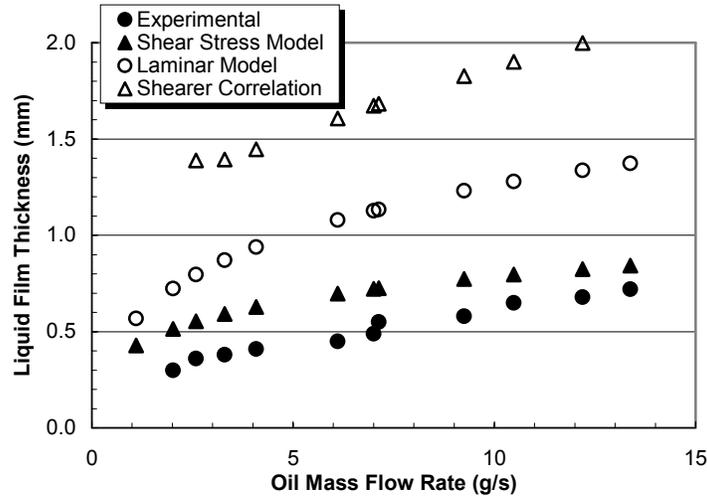
Figure 6. Comparison of Oil Film Thickness between Different Models and Experimental Data
