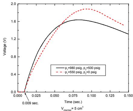
Figure 8: Comparison of filling behaviors for similar pressure differences, but with different  $p_1$ s.
