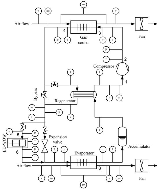
Figure 13: Experimental setup of transcritical CO<sub>2</sub> cycle with ED-WOW
