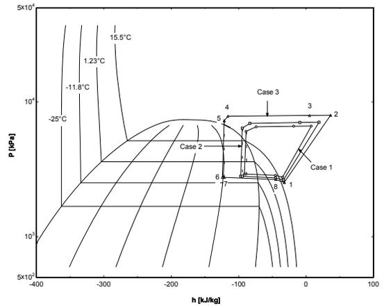
Figure 15: Pressure-enthalpy diagram of the system processes.
