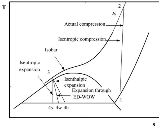
Figure 2: Temperature-entropy diagram of transcritical carbon dioxide cycle.
