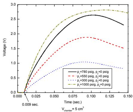
Figure 7: Filling behaviors of CO<sub>2</sub> in the chamber with the intake valve ( $D_{\text{orifice}}=3/64$  in).
