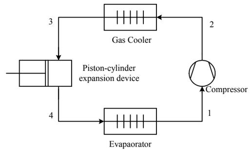
Figure 5: Schematic of transcritical CO<sub>2</sub> cycle with piston-cylinder expansion device replacing expansion valve.
