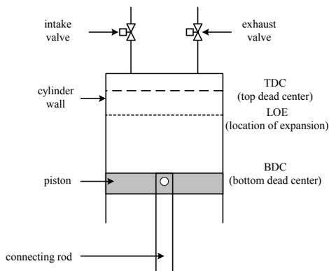
Figure 3: Piston-cylinder device with the related components and piston positions.
