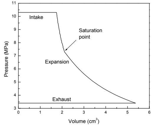
Figure 4: Piston processes with assumption of ideal process.
