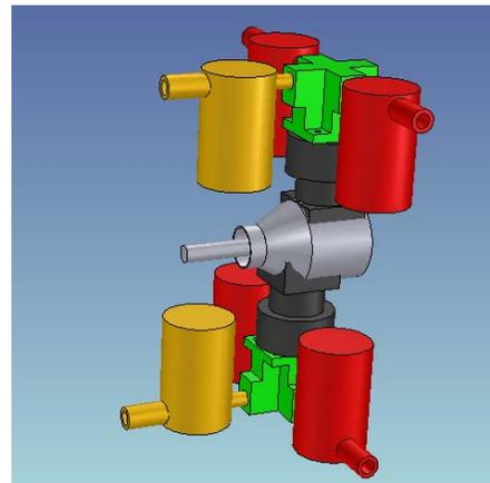
Figure 11: Assembly of Piston-cylinder work extraction expansion device.
