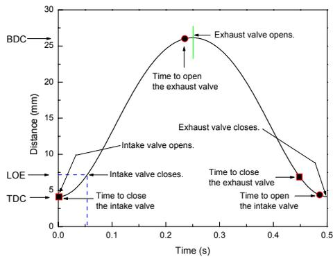
Figure 9: Timings for input signals to the solenoid valves.
