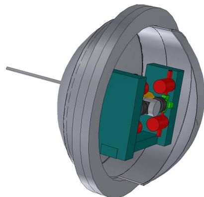
Figure 12: Cut view of the designed enclosure with expansion device in scale.
