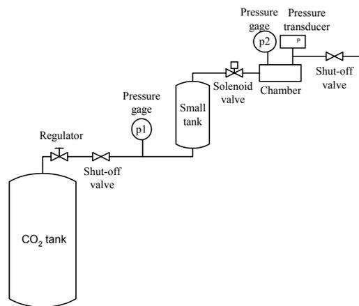
Figure 6: Schematic of test stand to determine the opening time of the intake valve.
