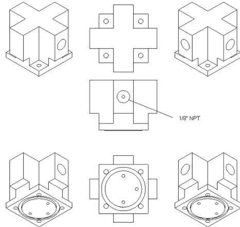
Figure 10: Several views of the head of the piston-cylinder device.
