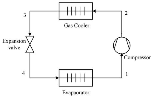
Figure 1: Schematic of basic transcritical carbon dioxide cycle.
