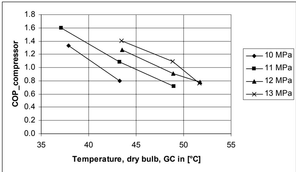
Figure 4: Coefficient of Performance
