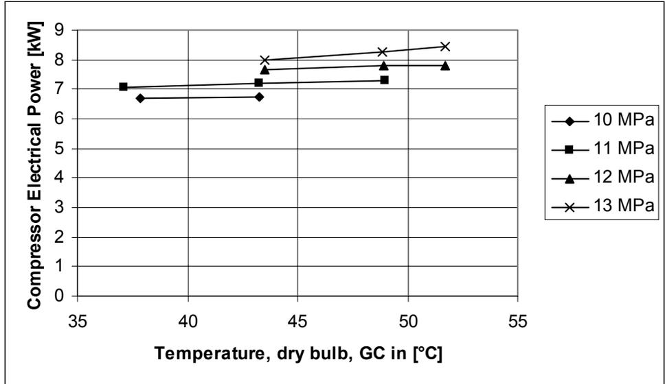
Figure 3: Compressor electrical power
