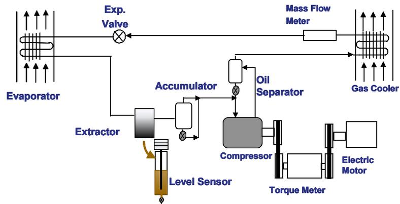
Figure 1 CO<sub>2</sub> Automotive Air-Conditioning System
