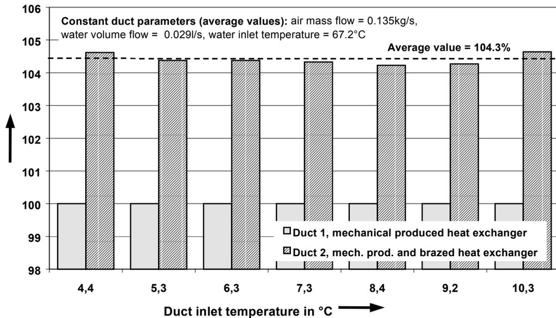
Figure 3: Long term test, capacity transfer (water side) for different duct inlet temperatures and heat exchangers
