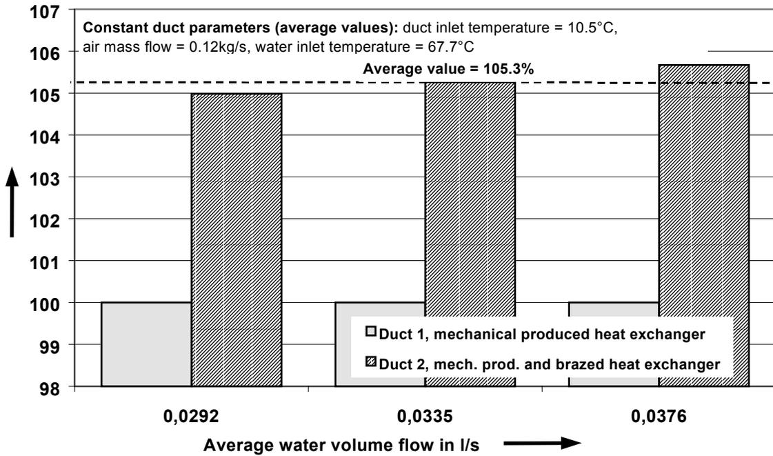
Figure 4: Short term test, capacity transfer on the water side for different average water volume flows and heat exchangers
