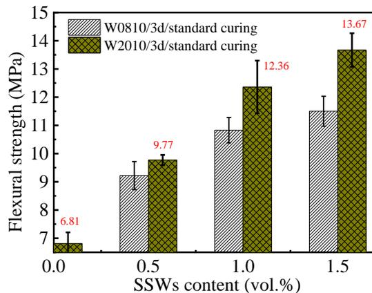
Fig. 1 Flexural strength of SSWs reinforced RPC
