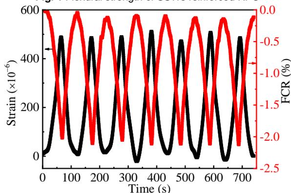
Fig. 2 Self-sensing property of RPC with SSWs in diameter of 8  $\mu\text{m}$  and volume fraction of 1.0 vol.% under cyclic compressive
