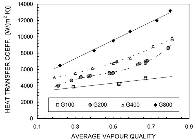
Figure 2: Heat transfer coefficients for R134a at  $40^\circ\text{C}$  saturation temperature. G is mass velocity [ $\text{kg}/(\text{m}^2 \text{ s})$ ].
