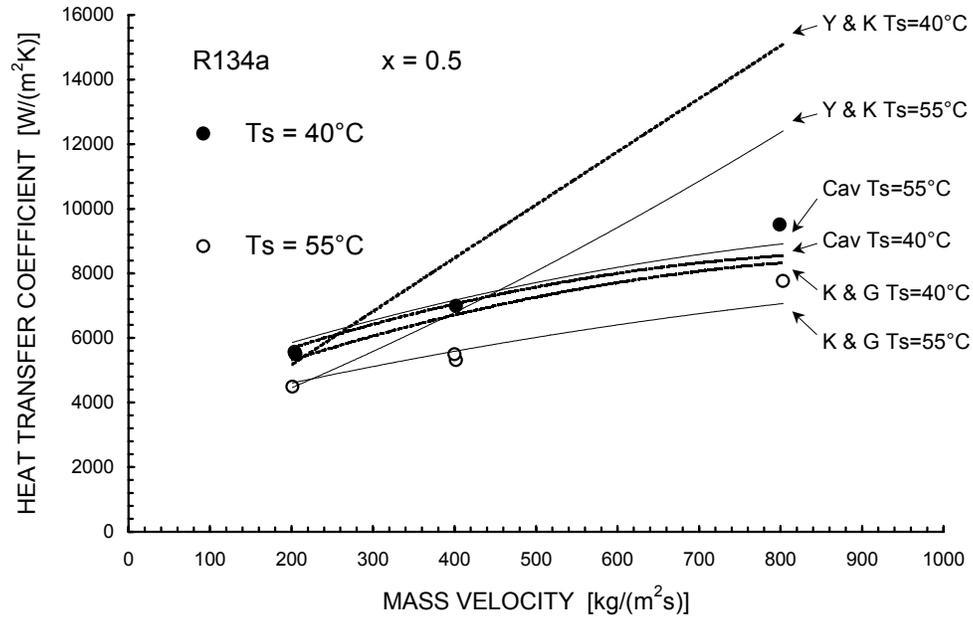
Figure 8: Experimental (markers) and calculated (lines) heat transfer coefficients for R134a at 40°C and 55°C saturation temperature. The following models are applied: Cavallini et al. (1999) [Cav], Kedzierski and Goncalves (1997) [K & G] and Yu & Koyama (1998) [Y & K].
