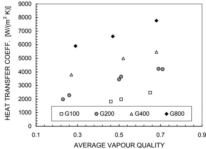
Figure 6: Heat transfer coefficients for R407C at 55°C average saturation temperature.
