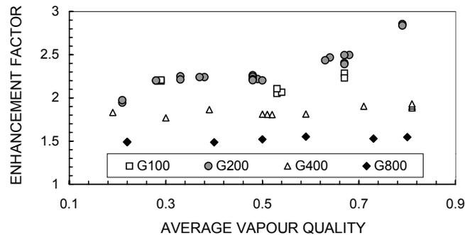
Figure 3: Heat transfer enhancement factor for R134a at  $40^\circ\text{C}$  saturation temperature.
