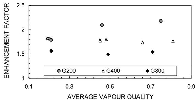
Figure 5: Heat transfer enhancement factor for R134a at 55°C saturation temperature..
