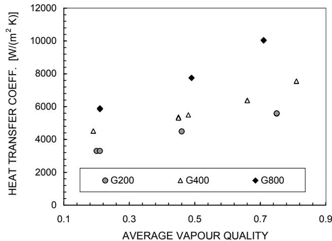
Figure 4: Heat transfer coefficients for R134a at 55°C saturation temperature. G is mass velocity [kg/(m<sup>2</sup>s)].
