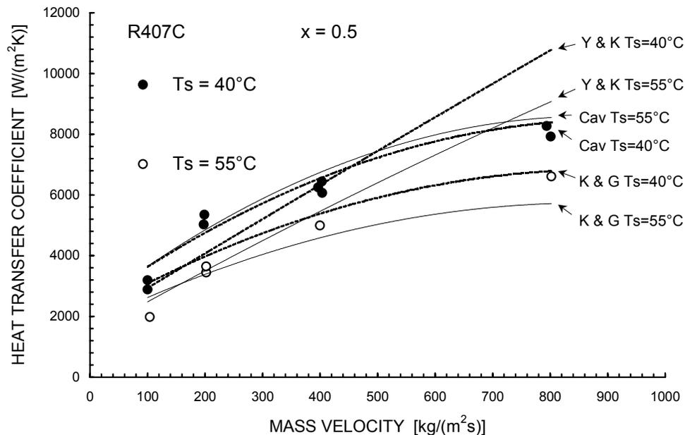
Figure 9: Experimental (markers) and calculated (lines) heat transfer coefficients for R407C at 40°C and 55°C saturation temperature. The following models are applied: Cavallini et al. (1999) [Cav], Kedzierski and Goncalves (1997) [K & G] and Yu & Koyama (1998) [Y & K]. All these three models are applied along with the Bell and Ghaly correction (1973).
