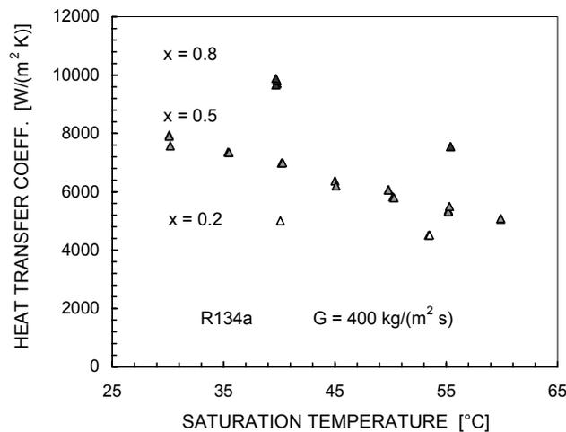
Figure 7: Experimental heat transfer coefficients for R134a at varying saturation temperature.
