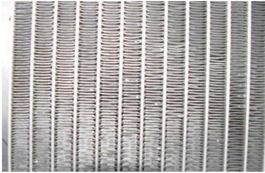
Figure 1: Remaining condensate in the vertically placed microchannel heat exchanger with 15 FPI after a defrost cycle
