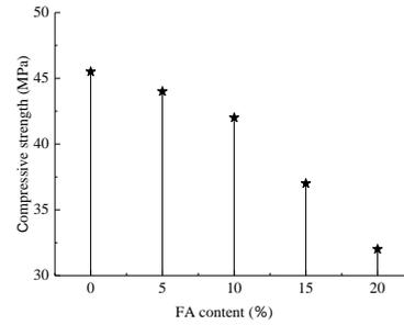
**Figure 1.** Compressive strength of MPC with different FA content at 28 day
