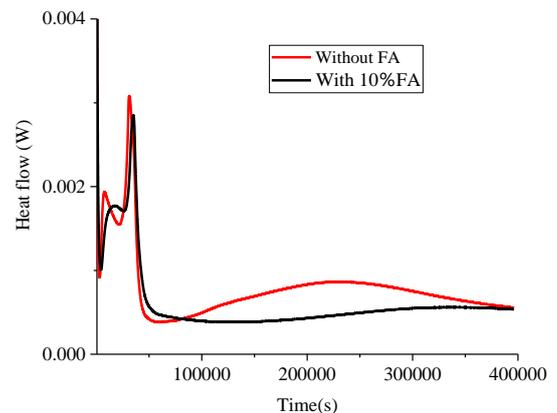
**Figure 2.** Hydration heat release rate of MPC
