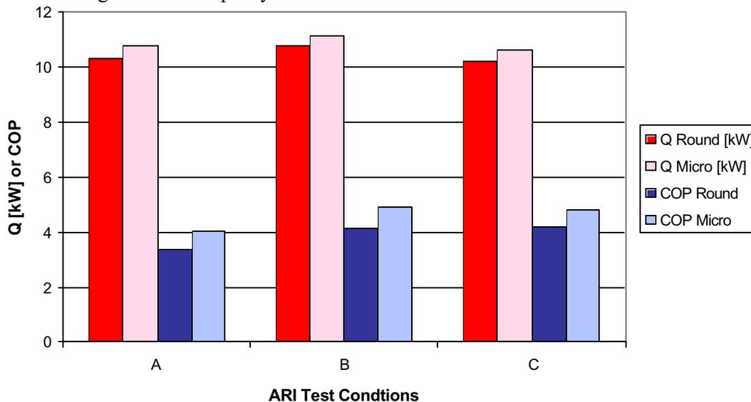
Fig. 5. Comparison of system data - capacity  $Q$  and coefficient performance (COP) - for the same system with the round-tube condenser and the microchannel parallel-flow condenser under ARI condition A, B, and C. The air-flow rate was the same.
