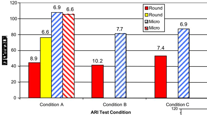
Fig. 17. ARI conditions A, B, and C: overall heat-transfer coefficients in the microchannel and the round-tube condensers. The values on the bar represent subcooling under each condition.
