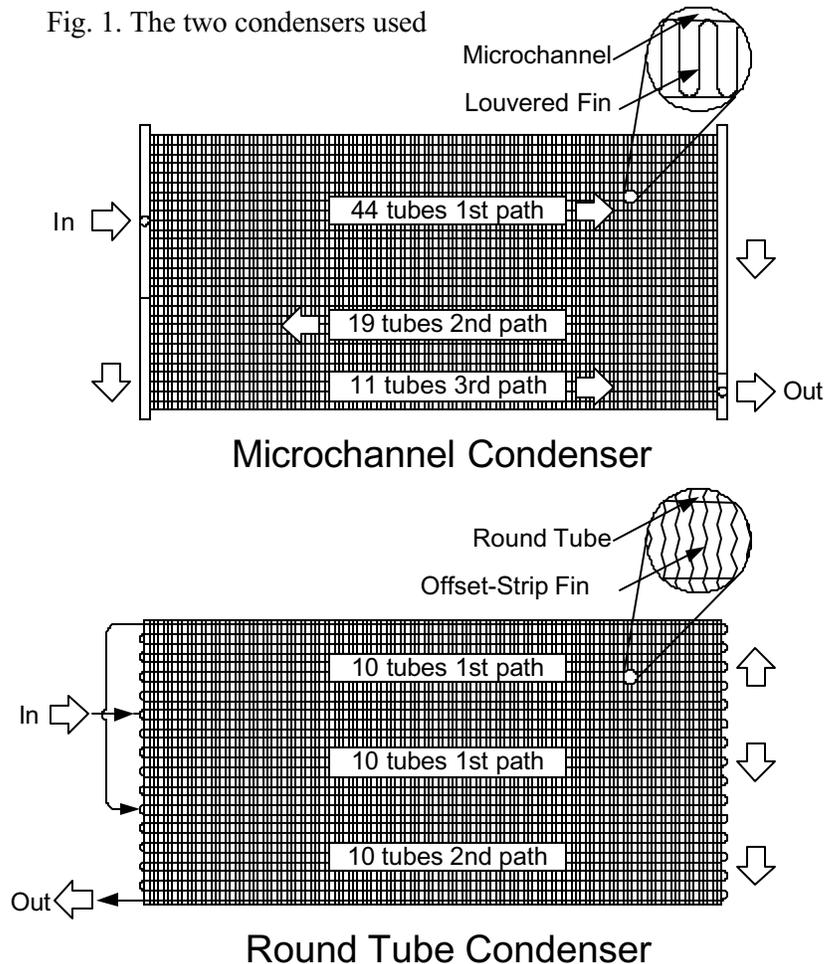
Fig. 2. Schematics of the unfolded condensers.
