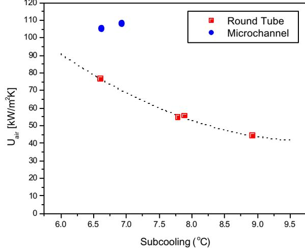
Fig. 18. Overall heat-transfer coefficients in the microchannel and the round-tube condensers under certain subcooling conditions
