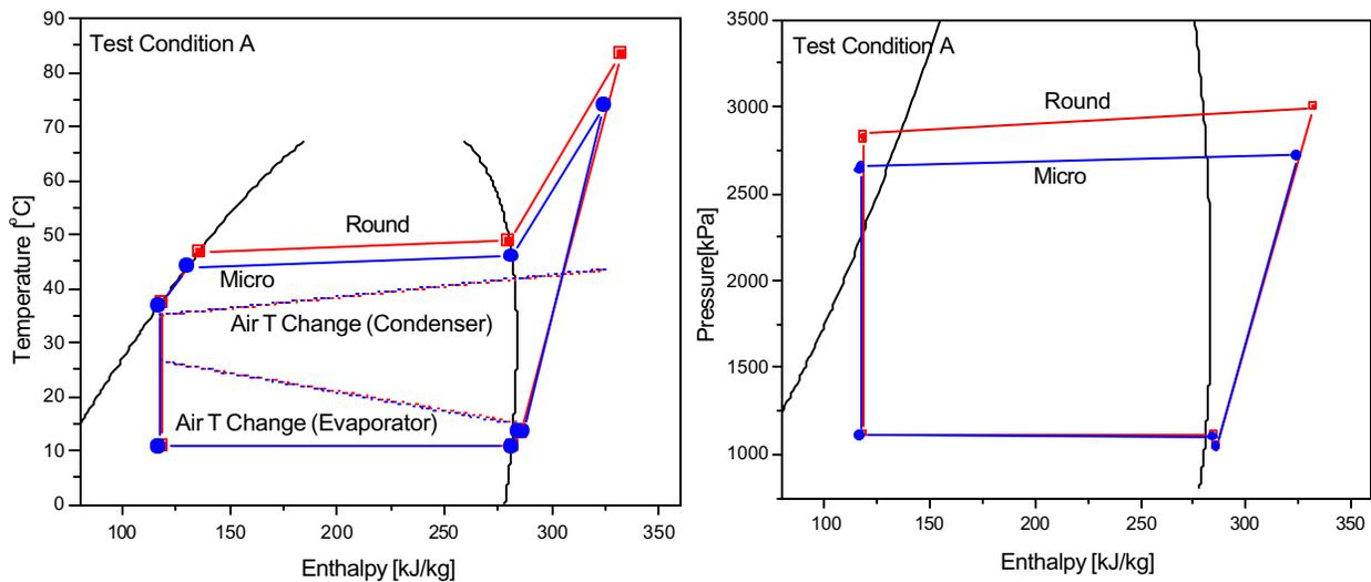
Fig. 7. Cycle comparison: ARI condition A, effect of two condensers on systems
