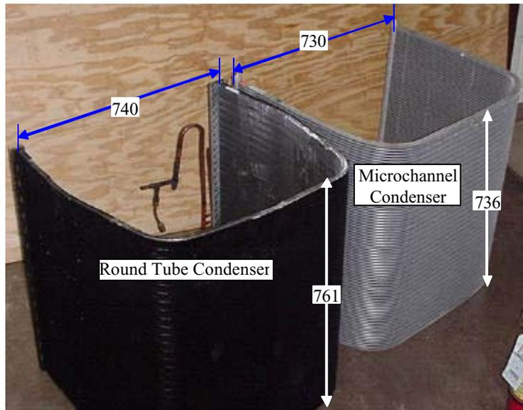
Fig. 1. The two condensers used
