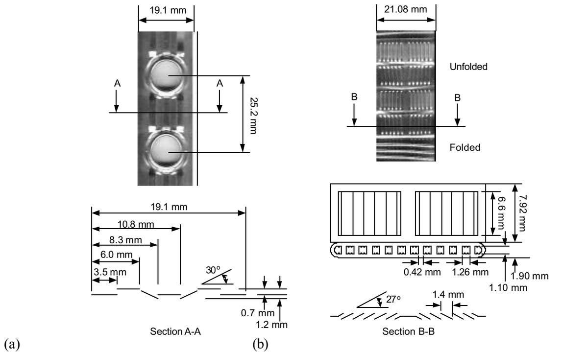
Fig. 3. (a) Offset-strip fins for the round-tube condenser, (b) Louver folded fin and microchannel dimension used in the microchannel condenser.
