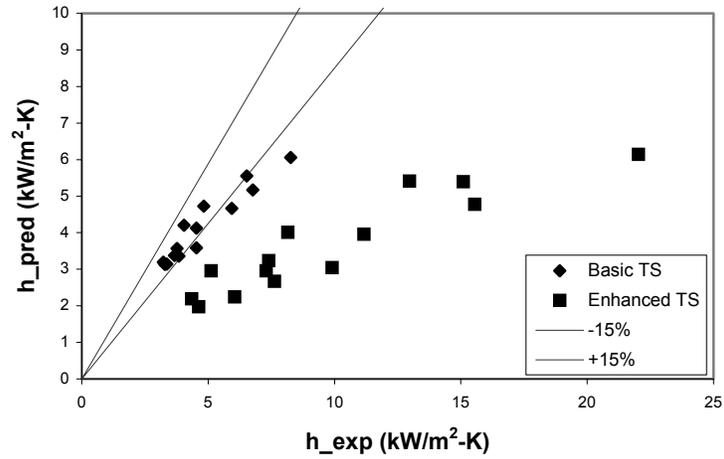
Figure 9: Comparison of Wattelet (1994) Heat Transfer Correlation with Experimental Results
