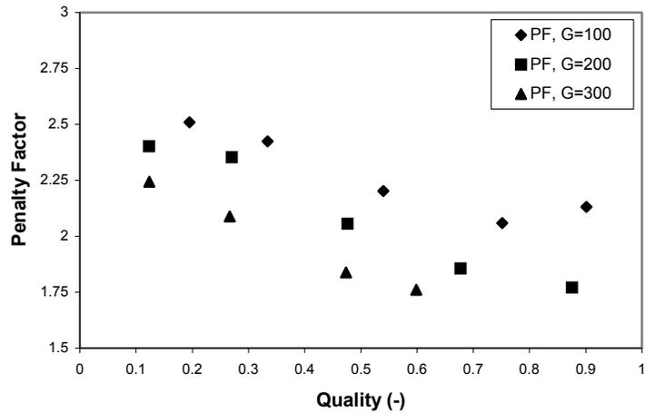
Figure 8: Penalty Factors for Basic and Enhanced Test Sections (Mass Flux, G in kg/m<sup>2</sup>s)
