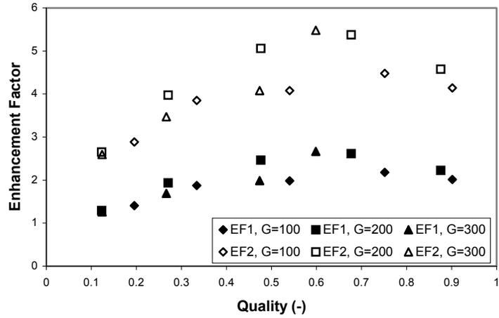
Figure 6: Enhancement Factors for Basic and Enhanced Test Sections (Mass Flux, G in kg/m<sup>2</sup>s)
