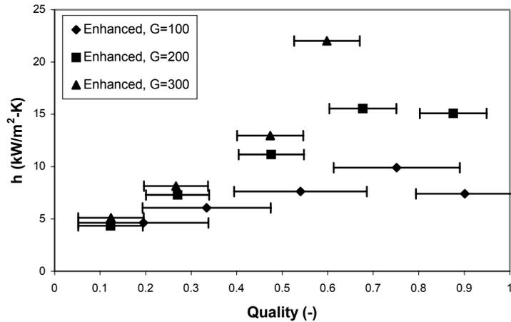
Figure 5: Enhanced Test Section Heat Transfer Coefficients (Mass Flux, G in kg/m<sup>2</sup>s)
