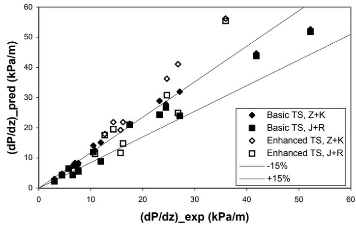
Figure 10: Comparison of Zhang and Kwon (1999) and Jung and Radermacher (1989) Pressure Drop Correlations with Experimental Results
