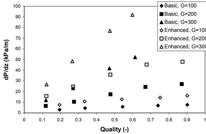
Figure 7: Pressure Drop Data for Basic and Enhanced Test Sections (Mass Flux, G in kg/m<sup>2</sup>s)
