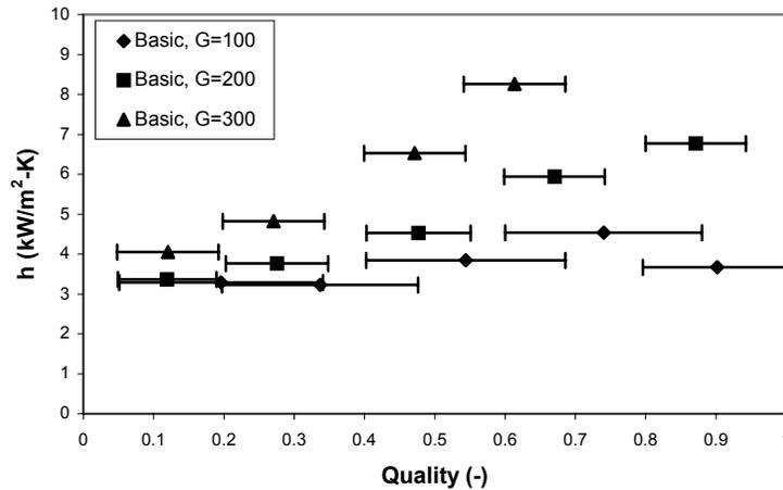
Figure 4: Basic Test Section Heat Transfer Coefficients (Mass Flux, G in kg/m<sup>2</sup>s)
