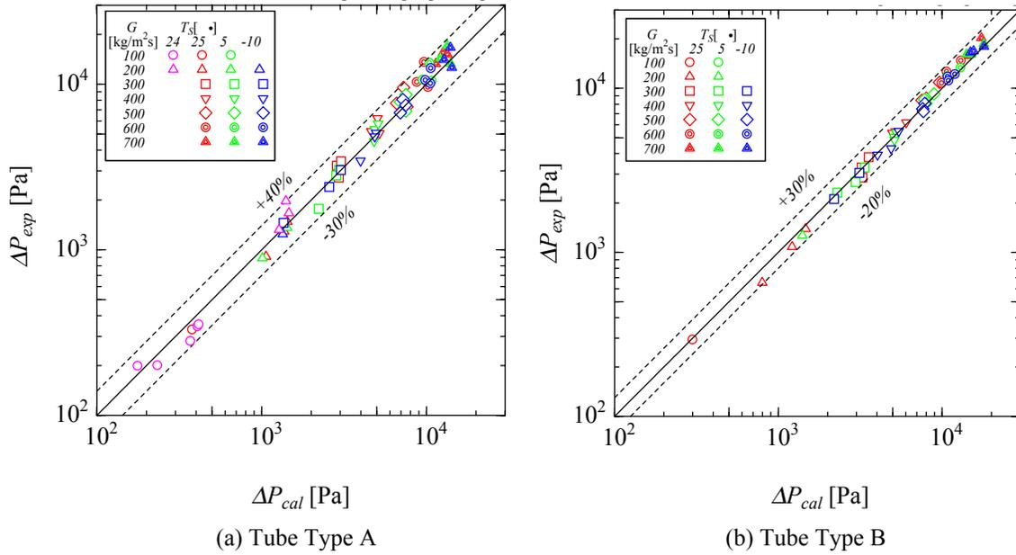
Figure 4: Comparison between measured and predicted pressure drop by equation (7).
