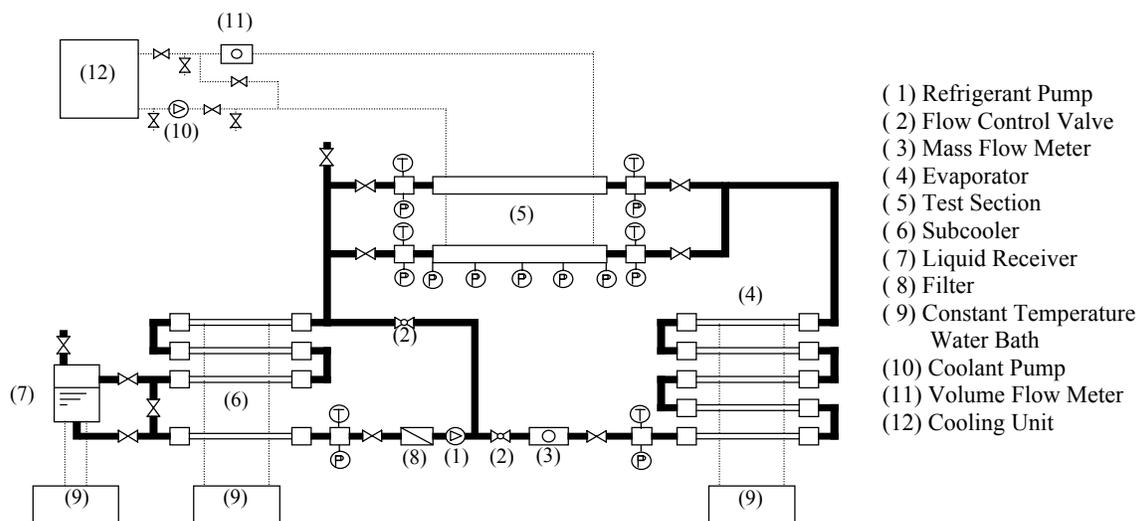
Figure 1: Schematic view of experimental apparatus.
