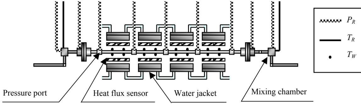
Figure 2: Schematic view of test section.
