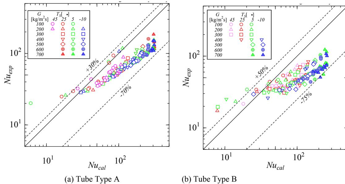
Figure 6: Comparison between experimental data and correlation of Haraguchi *et al.*
