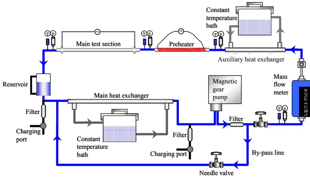
Figure 1: Schematic diagram of experimental apparatus for evaporative heat transfer test with a microtube.
