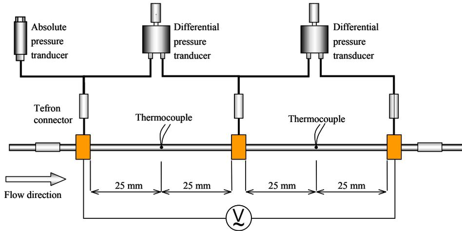
Figure 2: Representation of the measuring points in the test section.
