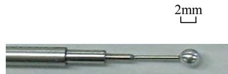
Fig.2 Measuring probe
