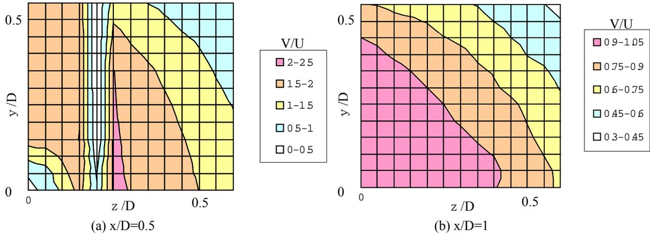
Fig. 4 Velocity contour of fan for representative streamwise locations
