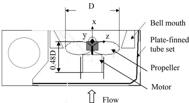
Fig.1 Flow field and coordinate system (Top view)
