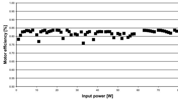
Figure 6; Motor efficiency versus the input power
