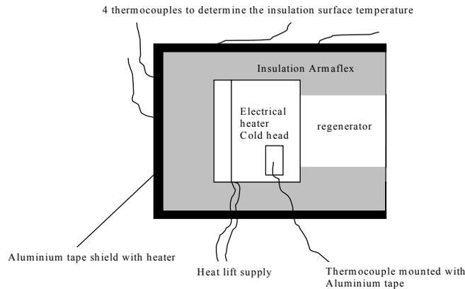
Figure 2; Cold head insulation covered with Aluminium tape
