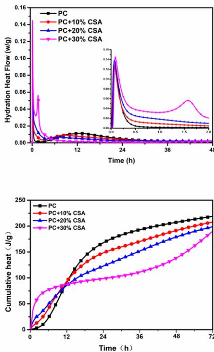
Fig. 2. Isothermal calorimetry data for PC-CSA binary system.
