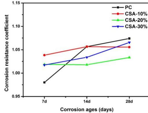
Fig.4 Compressive corrosion resistance coefficient of samples in 3.5% NaCl solution.
