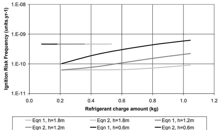
**Fig. 1: Results for units installed at different heights**
