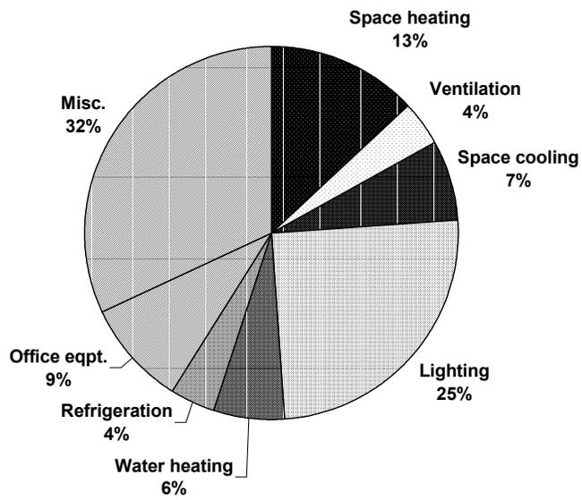
Figure 2. 1997 Primary Energy Consumption in U.S. Commercial Buildings
