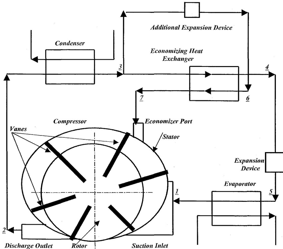
Figure 1: Schematic of a Refrigeration System with an Economizer Port
