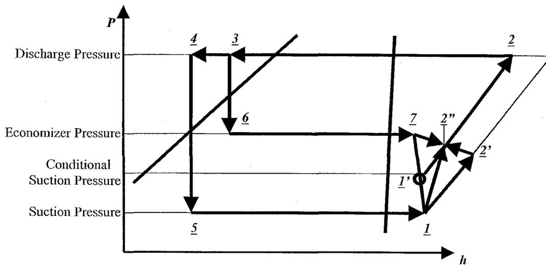
Figure 2: Economizer Cycle in P-h Diagram
