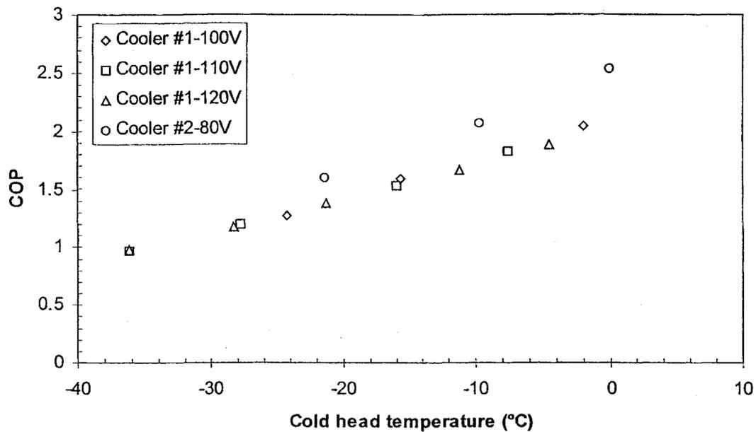
Figure 5. COP values for coolers #1 and #2 (Warm head temperature: 30°C)
