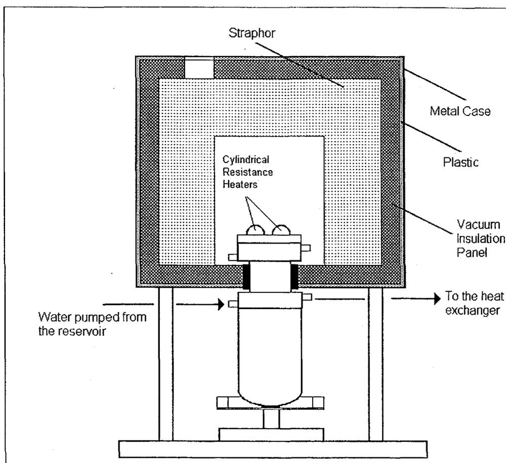
Figure 1. Schematic diagram of the so-called adiabatic box and the FPSC.
