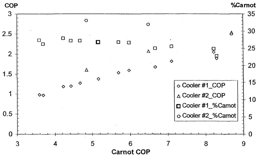
Figure 6. COP and Carnot Fraction for coolers #1 and #2.
