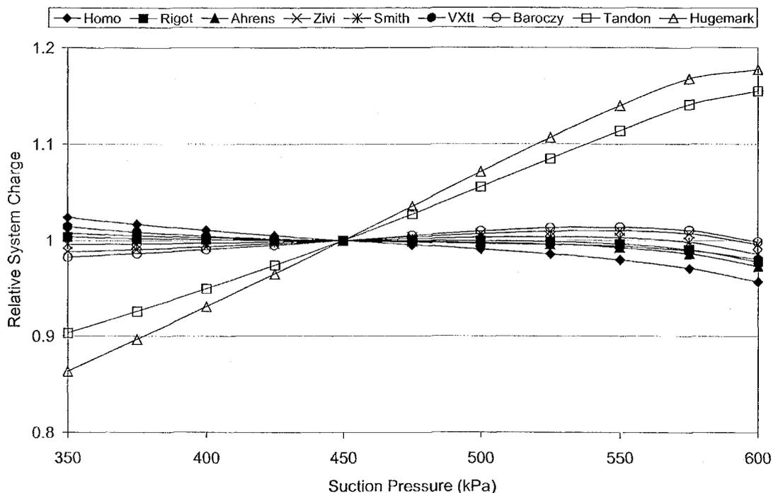
Figure 3 Effect of Suction Pressure on System Charge
