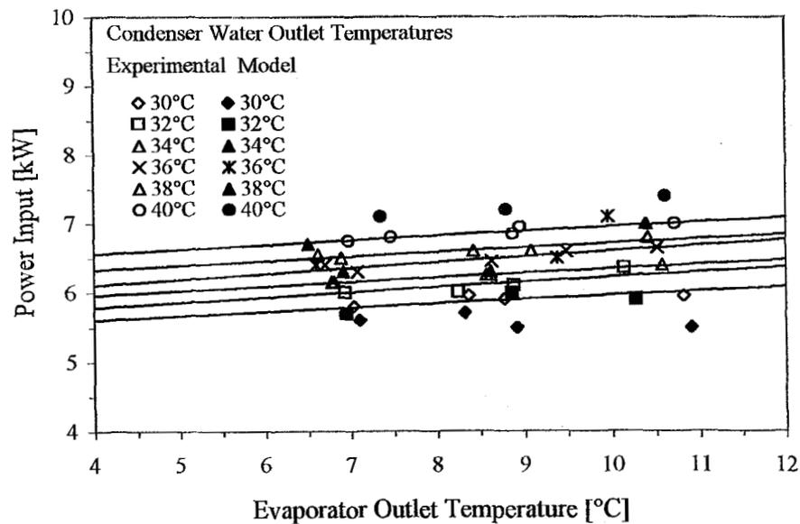
Figure 5 Steady-state power consumption
