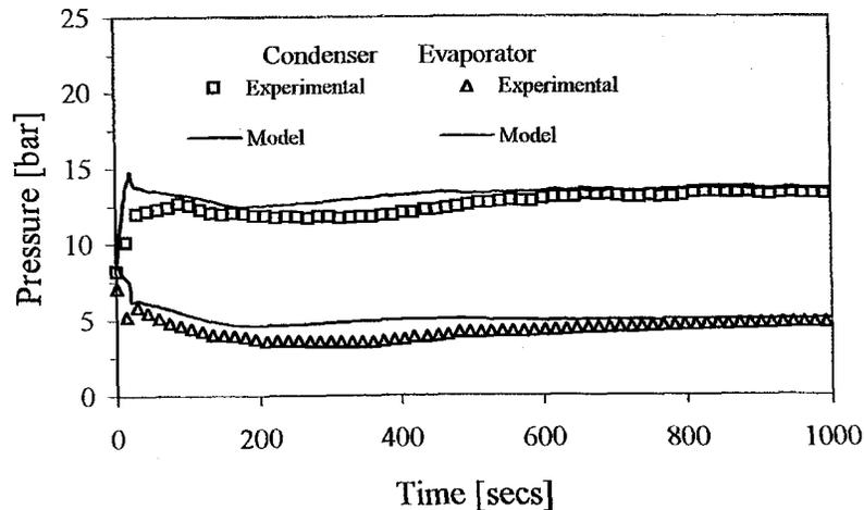
Figure 7 Start-up refrigerant pressures
