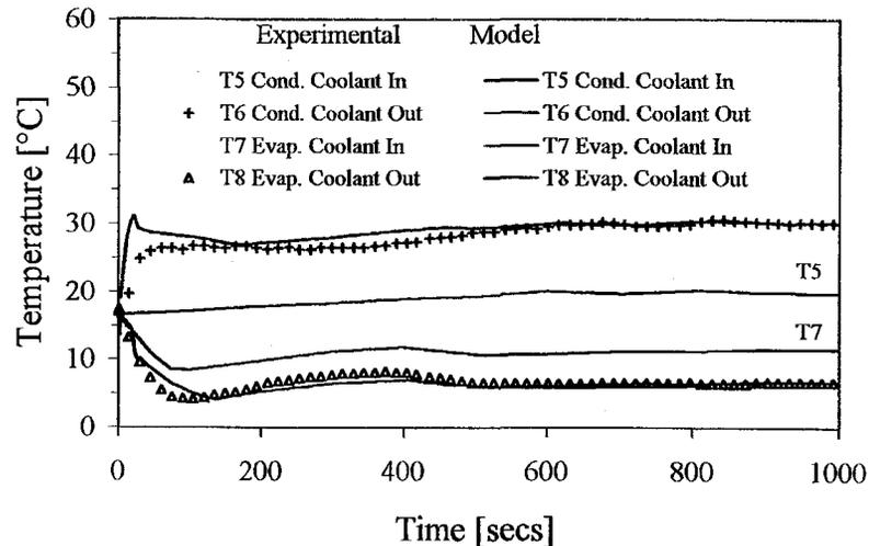
Figure 8 Start-up coolant temperatures
