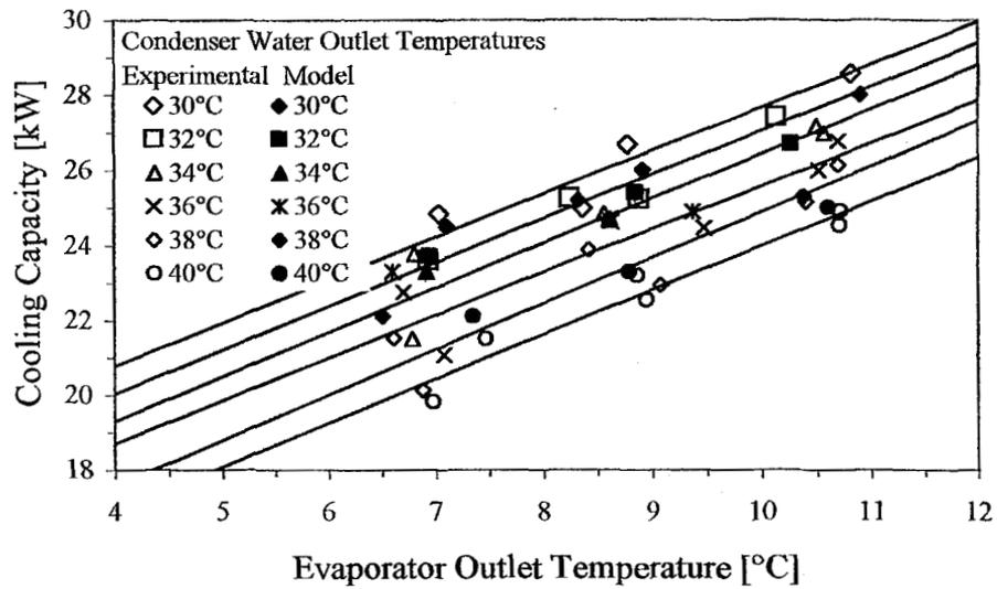
Figure 4 Steady-state cooling capacity
