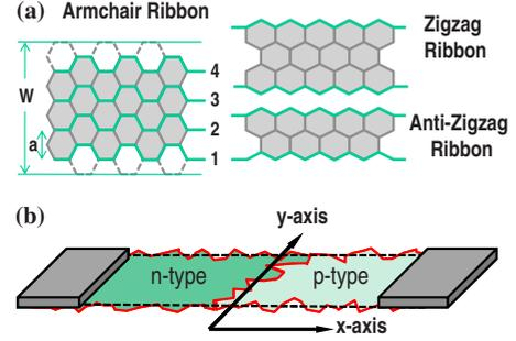
FIG. 1. (Color online) (a) Illustrations of armchair, zigzag, and anti-zigzag edge ribbons. The carbon layer numbering convention for an armchair edge ribbon used in this work is also depicted. (b) Schematic of the two terminal  $p$ - $n$  junction simulated in this work, illustrating also the ID and ED.
