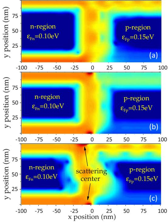
FIG. 4. (Color online) Intensity plot of the nonequilibrium electron density,  $\log_{10}(n)$ , for various ribbons with width  $\approx 100$  nm. We plotted for the case (a) armchair ribbon (no disorder) with 401 carbon layers along the width, (b) zigzag ribbon (no disorder), and (c) zigzag ribbon (with interface disorder). The magnetic field is assumed to be 10 T, while the depletion width 25 nm.
