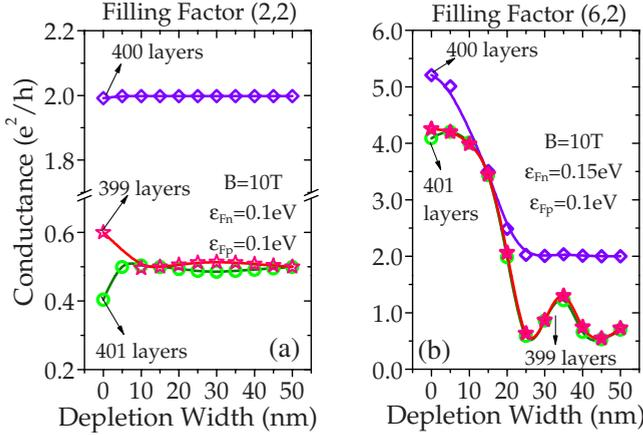
FIG. 3. (Color online) (a) Junction conductance as a function of depletion width in the clean limit, i.e., no disorder, for armchair ribbons of different widths for the case of filling factor (2,2). (b) Same as (a) excepts for filling factor of (6,2).
