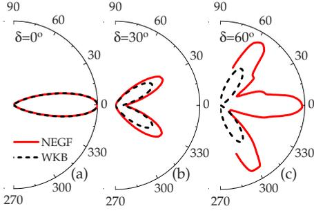
FIG. 3. (Color online) [(a)–(c)] Polar plots of the transmission probability  $T_{negf}(\theta_m) = \sum_n T_{negf}^{mn}$  for different  $\delta$ , where  $T_{negf}^{mn}$  is computed using the same device parameters as for Fig. 2. The WKB plots are obtained using the usual WKB formula (Ref. 13) (see text)
