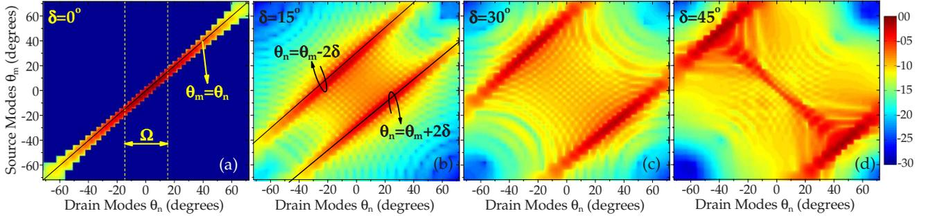
FIG. 2. (Color online) NEGF derived mode-to-mode transmission probability function  $\log_2[T_{negf}(\theta_m, \theta_n)]$  for a symmetric  $p$ - $n$  junction device biased at  $\epsilon_f=0.4$  eV, for tilt angles of  $\delta=0^\circ, 15^\circ, 30^\circ, 45^\circ$ , respectively. The device width is 100 nm and the  $p$ - $n$  transition length  $D=10$  nm.
