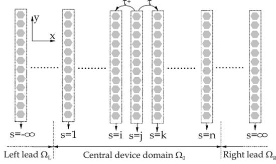
FIG. 7. Schematic on a graphene ribbon with armchair edges. Each slice of supercell consist of an intracell interaction denoted by  $\alpha$  and a right/left neighboring-cell interaction represented by  $\tau/\tau^\dagger$ , respectively.
