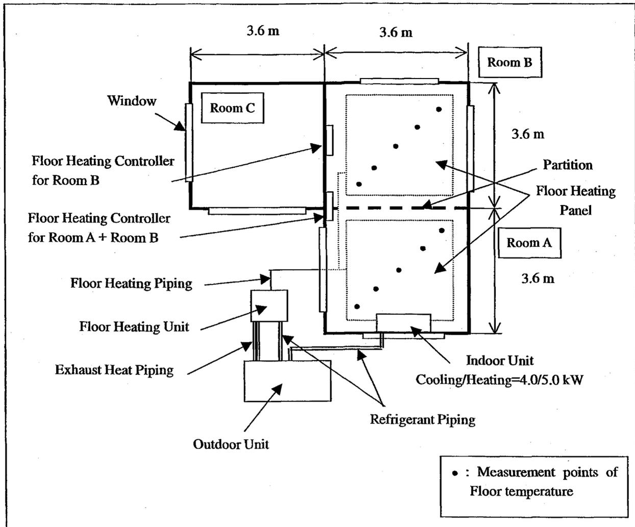
**Figure 4.** Layout of Laboratory for the Environmental Experiment (Overview)
