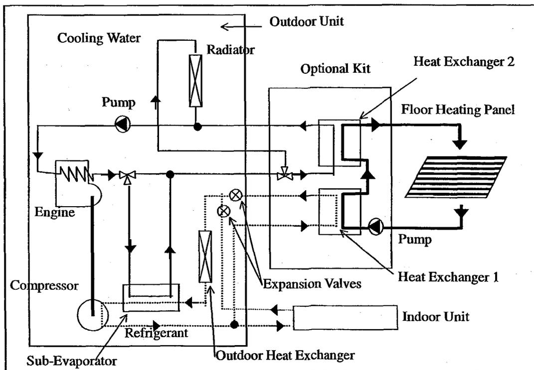
Figure 3. Schematic Diagram of the Floor Heating System
