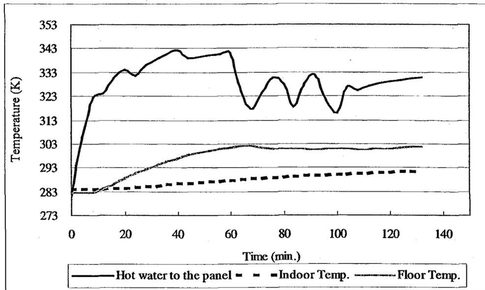
**Figure 5. Trend of the Temperature of Floor Heating System using GHP**
