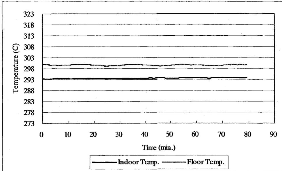
Figure 6. Trend of Temperature of Floor Heating System using GHP after Reaching the Steady State
