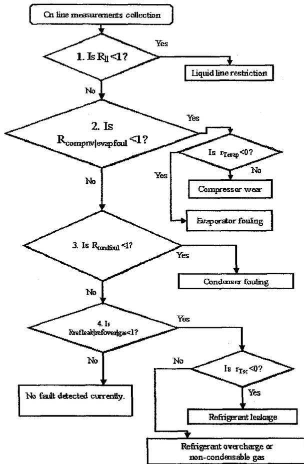
Figure 4 Sensitivity Ratio Method flowchart
