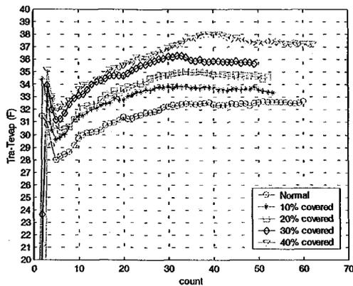
Figure 6 Evaporator fouling at  $T_{amb}=90F$
