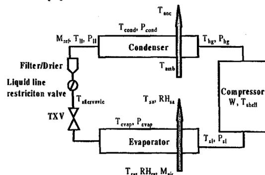
Figure 1 Test unit instrumentation
