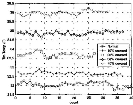
Figure 7 Evaporator fouling at  $T_{amb}=105F$
