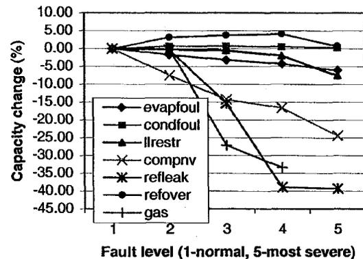
Figure 3 Impacts of faults on cooling capacity
