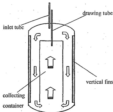
Figure 1 The schematic of the cryogenic PH<sub>3</sub> trapper
