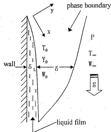
Figure 2 The schematic of condensation of liquid film
