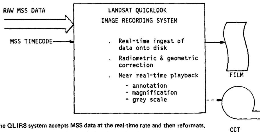
FIGURE 2. The QLIRS system accepts MSS data at the real-time rate and then reformats, corrects and outputs the full-resolution data at less than real-time rate.
