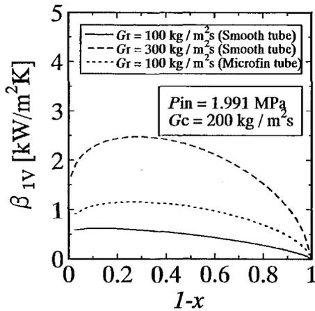
Fig. 4 Vapor mass transfer coefficient of component 1
