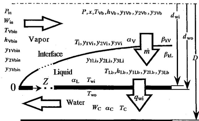
Fig.1 Physical model of double-tube condenser
