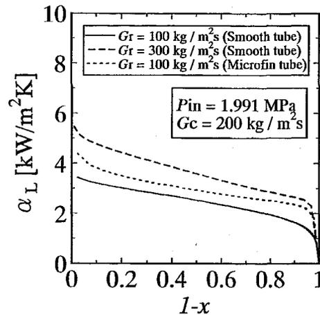
Fig. 5 Liquid heat transfer coefficient
