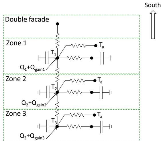
Fig. 1. Purdue Living Lab office room multi-zone thermal network structure
