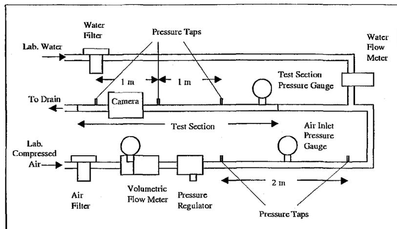
Figure 1: Experimental air/water test loop.
