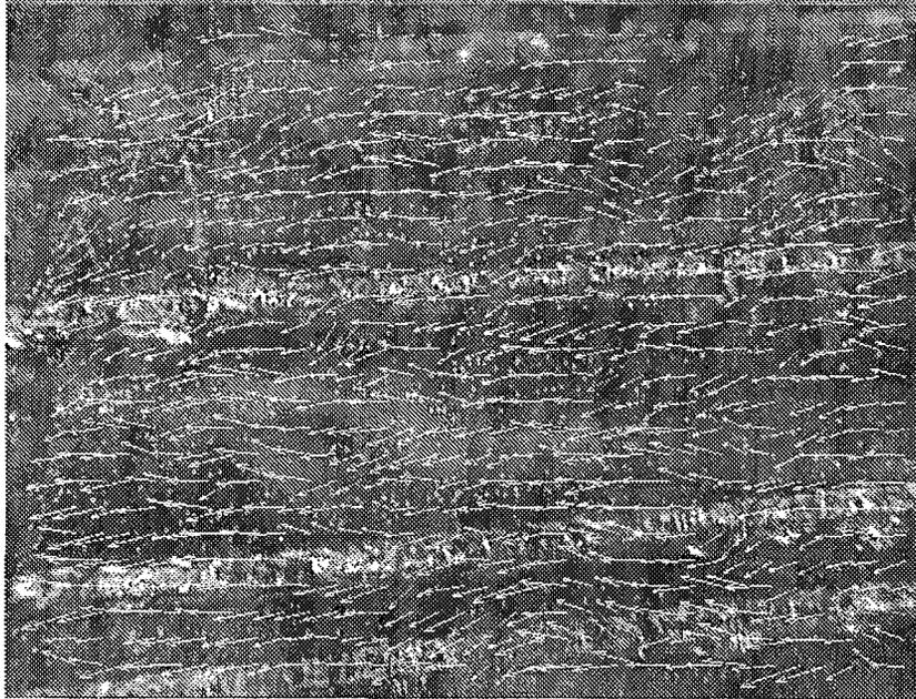
Figure 6: Local liquid film velocities 30 ms after the previous image was taken. The mean velocity to the left is approximately 0.1 m/s.
